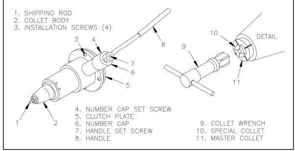
Figure 1. Quick Chuck features
